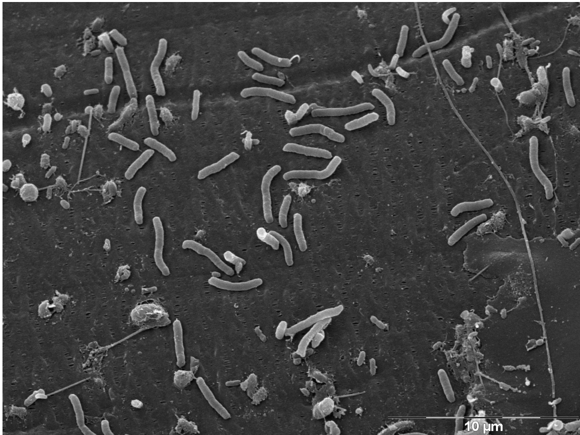
Figure 28. Scanning electron microscope image of biomass attachment on polypropylene membrane surface, 5000x magnification
